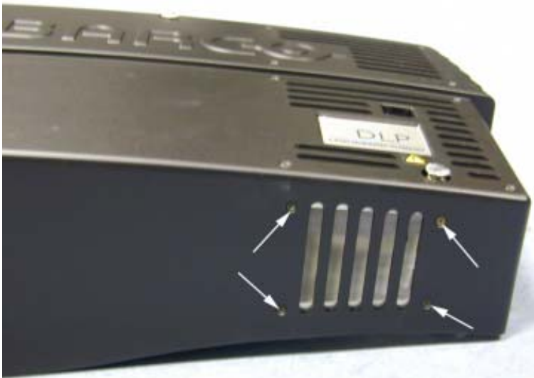
Image B-8 Dust filter removal
